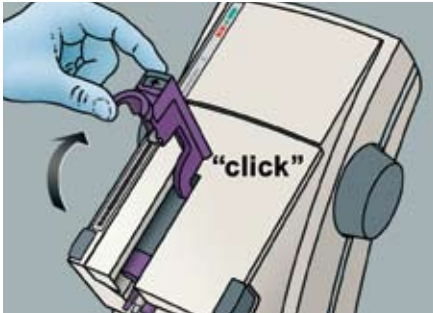
Fig. 9 Locking lever snaps into the uppermost position.
